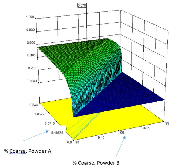
Fig. 1 FED output of two variables showing that less coarse powders are desirable in this application.
